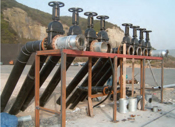
Spigot fitting for Gas and water supply
