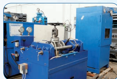
HYDRO - PNEUMATIC TEST UP TO 1000 bar
