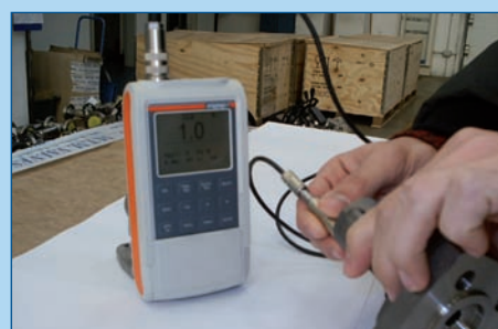
FERRITSCOPE FISHER FOR FERRITE DETERMINATION
