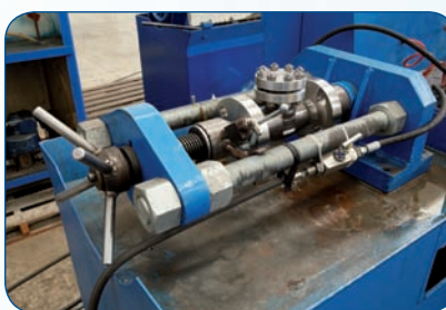
HYDRO - PNEUMATIC TEST UP TO 600 bar FOR CHECK VALVES
